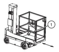
Figure 3-11. Traversing Platform
