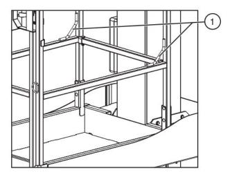
Figure 3-5. Lanyard Attachment Anchorage
