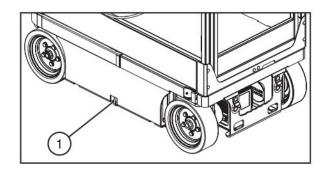
Figure 3-3. Pothole Protection Device
