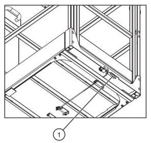
Figure 3-4. Platform Maintenance Lock
