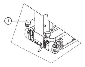
Figure 3-6. Flashing Light
