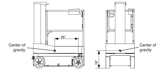
Figure 3-9. Center of Gravity
